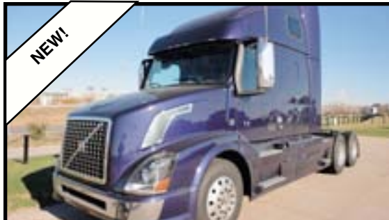
NEW! 2012 VOLVO VNL64T670 - Volvo D13 455 HP Eng, Eng Brake, 10 Spd, Air Ride Susp, 3.36 Ratio, 217" WB, 22.5LP Tires, Polished Alum Wheels, 61" Tandem Axle, 13,200 # FA, 40,000 # RA, Stk # 157740
