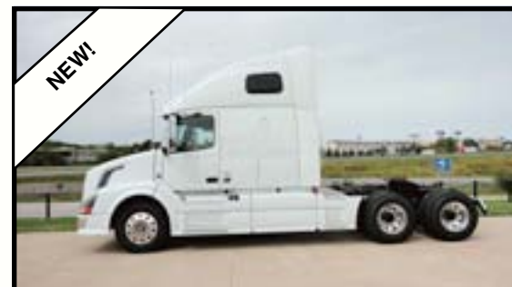
NEW! 2012 VOLVO VNL64T670 - Volvo D13 475 HP Eng, Eng Brake, 10 Spd, 4-Bag Air Ride Susp, 3.36 Ratio, 217" WB, 22.5LP Tires, Polished Alum Wheels, 61" Tandem Axle, 12,500 # FA, 40,000 # RA, Call for Pricing!!!! Stk #157545
